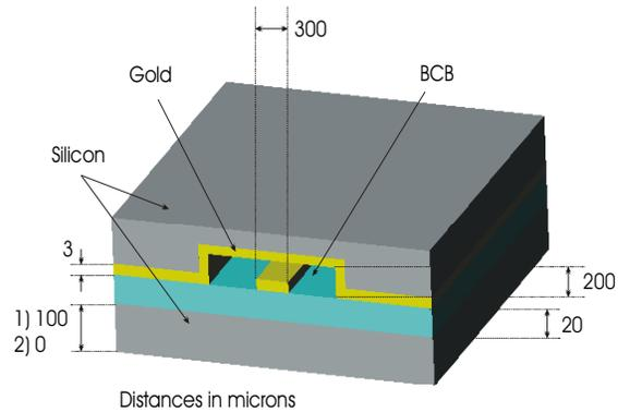
Figure 3. Inverted microstrip, taken from [5]
