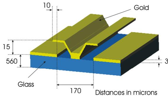
Figure 13. Coplanar transmission line over A glass substrate, taken from [16]
