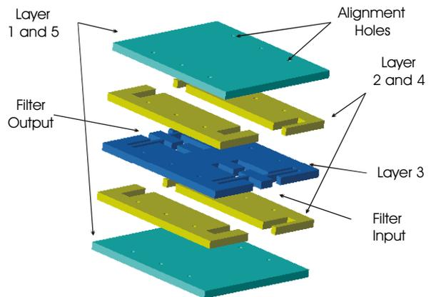
Figure 8. Suspended coaxial transmission line taken from [10]
