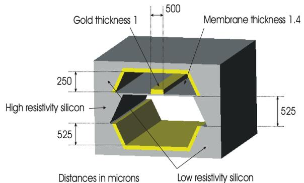
Figure 4. Microstrip over silicon membrane taken from [6]
