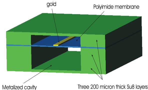
Figure 5. Microstrip over membrane using a SU8 shield, taken from [7]
