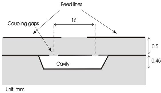
Figure 1. Cavity resonator at X band, taken from [2]
