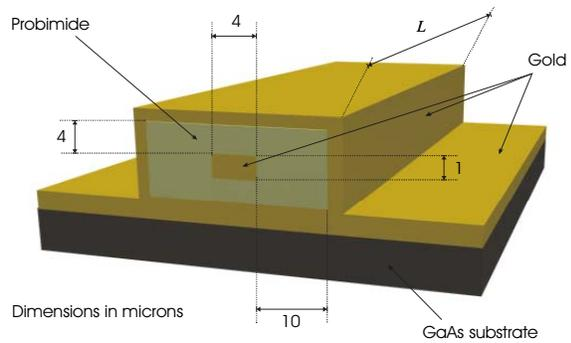
Figure 7. Dielectric filled coaxial transmission line taken from [9]
