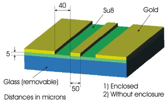
Figure 12. Coplanar transmission line over SU8 membrane, taken from [15]
