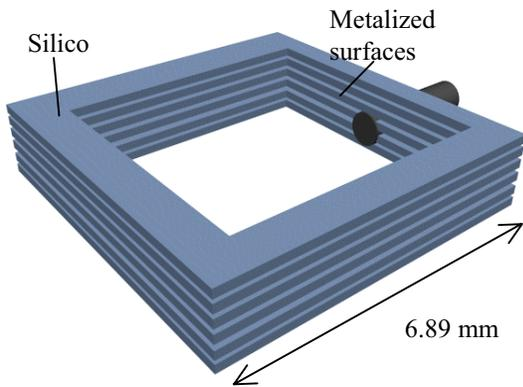
Figure 2. Micromachined silicon cavity without top cover, taken from [3]
