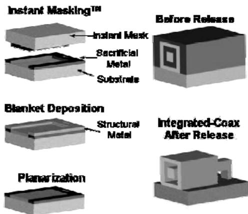
Figure 10. Process flow for the selective electrochemical metal deposition (EFAB™) taken from [13]
