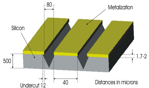
Figure 11. Coplanar micromachined transmission line taken from [14]
