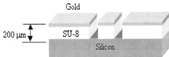
Figure 14. Coplanar transmission line on SU8 taken from [17]
