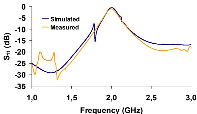
Fig. 7 Simulated and measured  $S_{11}$  (off state)
