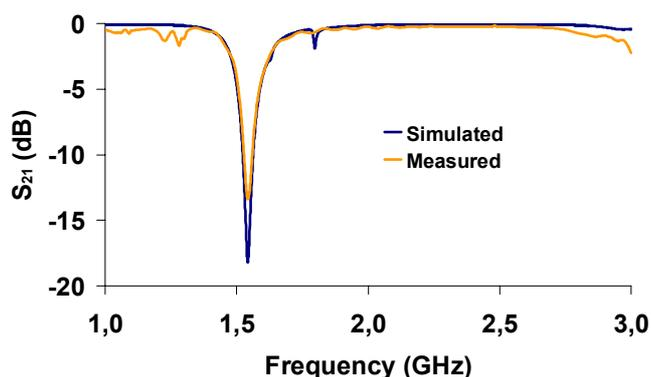
Fig. 8 Simulated and measured  $S_{21}$  (on state)
