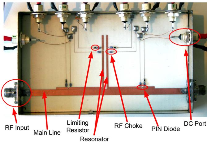
Fig. 5 Photograph of the switchable bandstop filter
