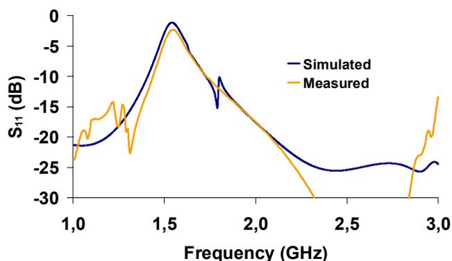
Fig. 9 Simulated and measured  $S_{11}$  (on state)
