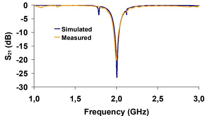
Fig. 6 Simulated and measured  $S_{21}$  (off state)
