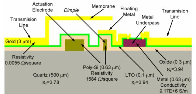
Fig. 3. Diagram of the cantilever MEMS switch on a quartz substrate.
