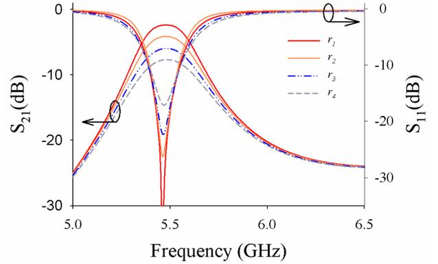
Fig. 6. Simulated results for different series cantilever MEMS switch contact resistance (ON state);  $r_1=1 \Omega$ ,  $r_2=10 \Omega$ ,  $r_3=20 \Omega$  and  $r_4=30 \Omega$ .
