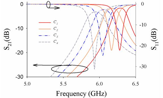
Fig. 7. Simulated results for different series cantilever MEMS switch capacitance (OFF state);  $C_1=1 \text{fF}$ ,  $C_2=10 \text{fF}$ ,  $C_3=20 \text{fF}$  and  $C_4=30 \text{fF}$ .
