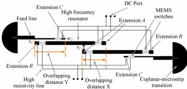
Fig. 1. Switchable bandpass filter topology.
