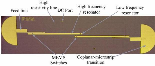
Fig. 4. Photograph of the switchable bandpass filter.
