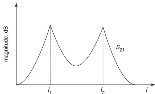
Fig. 5  $S_{21}$  simulated response for the dual-mode resonator
