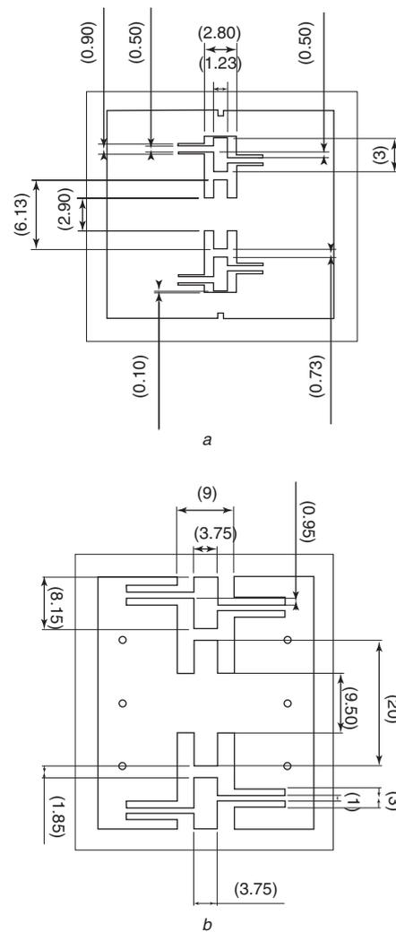
**Fig. 7** Dimensions of layer 3
