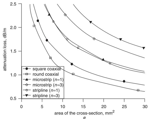
Fig. 3 Various different types of transmission line
