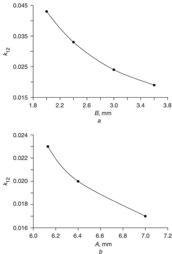
**Fig. 6** Coupling coefficient for the Ka-band filter
