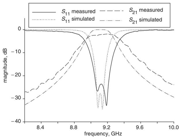
**Fig. 9** Response of the dual-mode X-band filter
