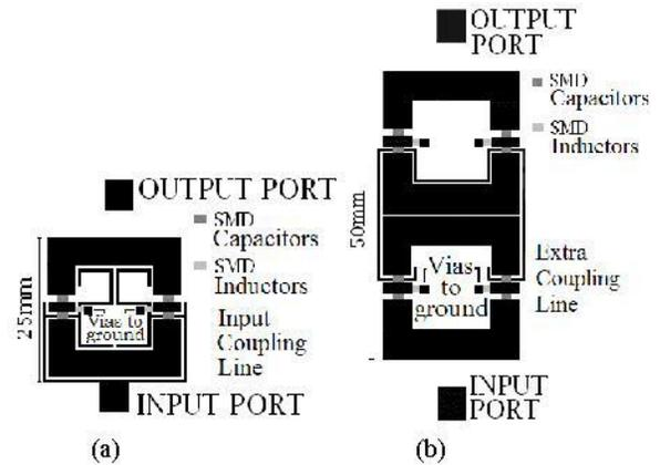
Fig. 2. Coupling configurations. (a) To achieve the desired  $Q_e$ . (b) To achieve the required  $k$  coupling.
