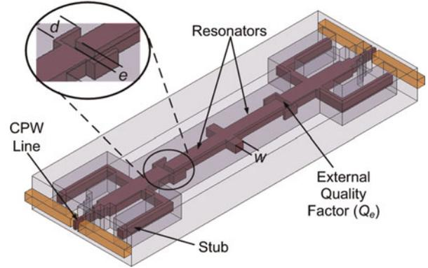
**Fig. 5.** 3D view of the U-band coaxial filter.
