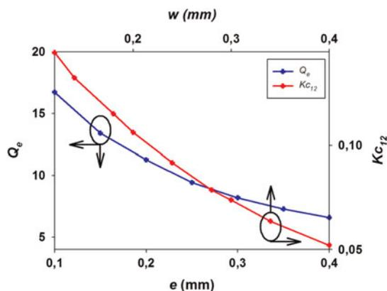
Fig. 8. External quality factor ( $Q_e$ ) and coupling coefficient ( $K_{C_{12}}$ ) for the V-band coaxial filter.
