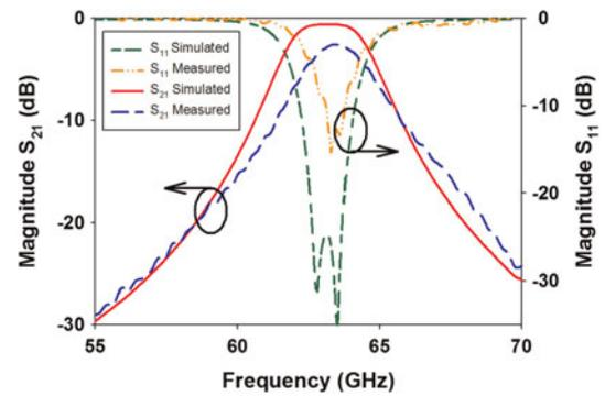
Fig. 9. Simulated and measured response for the V-band coaxial filter.
