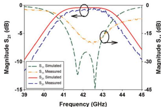
Fig. 7. Simulated and measured response of the U-band coaxial filter.
