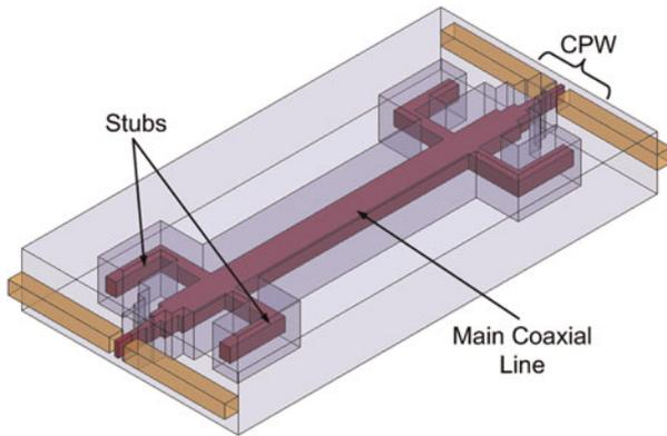
**Fig. 3.** 3D view of the CPW-to-coaxial line transition in a *back-to-back* configuration.
