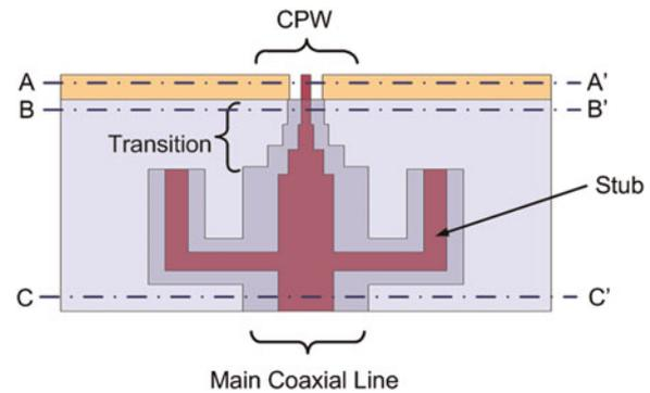
Fig. 1. Top view of the CPW-to-coaxial transition.
