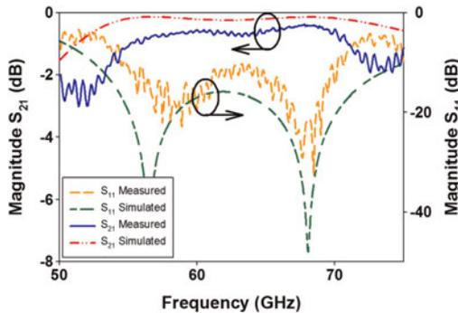
**Fig. 4.** Simulated and measured response of the suspended coaxial line.
