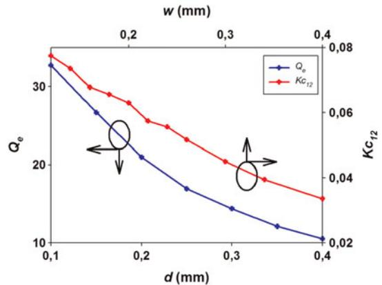
**Fig. 6.** External quality factor ( $Q_e$ ) and coupling coefficient ( $K_{C_{12}}$ ) for the U-band coaxial filter.
