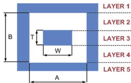
Fig. 2. Cross section of a rectangular coaxial line.
