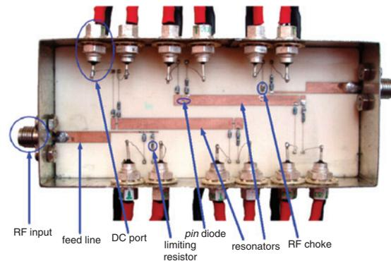
**Fig. 2** Photograph of switchable bandpass filter
