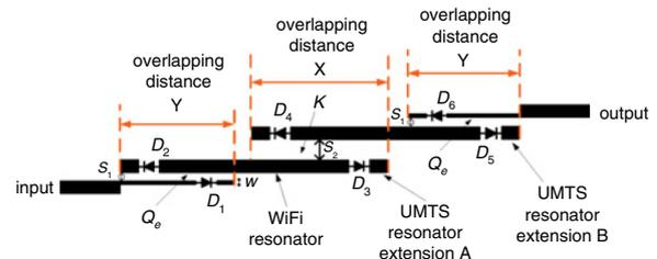
**Fig. 1** Switchable bandpass filter topology
