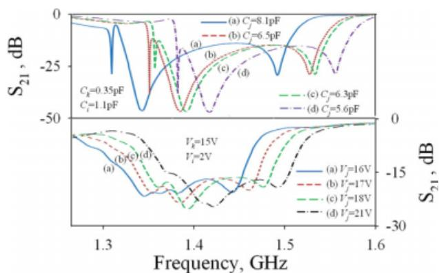
**Figure 5** Simulated and measured results for the band-stop filter with center frequency control (upper part: simulated response, lower part: measured response). [Color figure can be viewed in the online issue, which is available at [www.interscience.wiley.com](http://www.interscience.wiley.com)]
