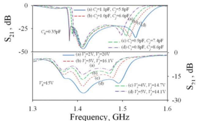
**Figure 6** Simulated and measured results for the band-stop filter with stopband bandwidth control (upper part: simulated response, lower part: measured response). [Color figure can be viewed in the online issue, which is available at [www.interscience.wiley.com](http://www.interscience.wiley.com)]
