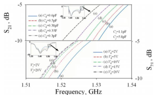
**Figure 7** Simulated and measured results for the band-stop filter with selectivity control (upper part: simulated response, lower part: measured response). [Color figure can be viewed in the online issue, which is available at [www.interscience.wiley.com](http://www.interscience.wiley.com)]
