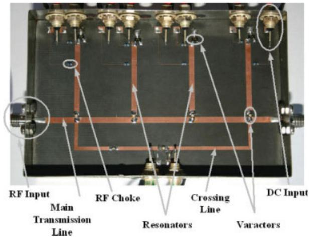
**Figure 4** Photograph of the reconfigurable quasi-elliptic band-stop filter. [Color figure can be viewed in the online issue, which is available at [www.interscience.wiley.com](http://www.interscience.wiley.com)]
