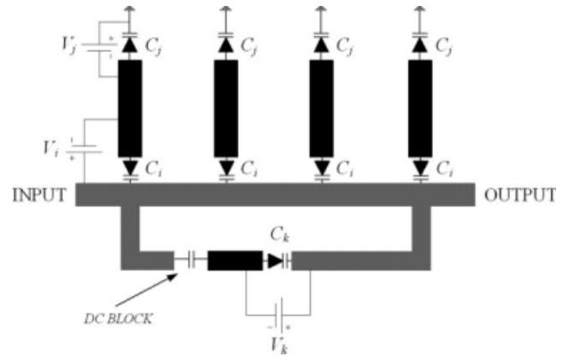
**Figure 3** Reconfigurable quasi-elliptic band-stop filter using varactor diodes
